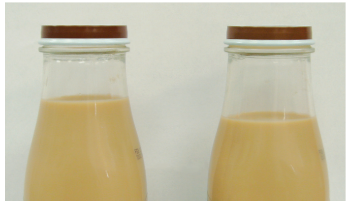
Full container (left), underfilled container (right).
